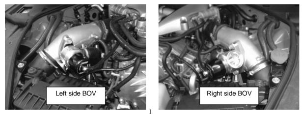
3) Replace the standard vacuum lines with the hose provided in each kit. Use the spring clamps to secure the lines.
