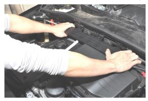
Unclip the 3 clips on the shroud and remove the wiring.
