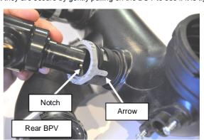
12) Make sure the orientation of the recirculation ports on the BOV's look like the picture below.
