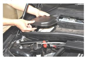
Pull the wiring harness cover towards the front of the car to slide it off the clips on the shroud
