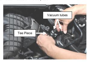
9) Remove the 2 standard bypass valves (BPV's) and their plumb back hoses by rotating the grey securing clips clockwise and pulling them out.
