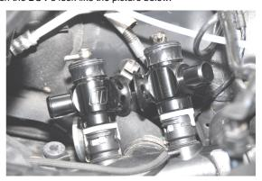
13) Install the recirculation hoses. Secure hoses with supplied hose clamps.
