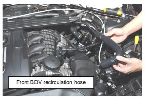
14) Connect the supplied vacuum tube to the tee piece and the Kompact BOV's. Secure the vacuum tube with the supplied hose clamps.
