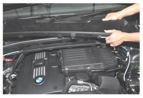
2) Remove ECU and brake distribution block cover by unclipping them off the shroud.
