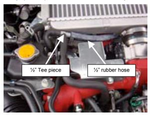
6. Push the plumb back side of the Turbosmart BOV onto the standard return pipe and secure the hose with the provided hose clamp. Unclip the hose shown in the picture from the bracket and move the line under the wiring loom that supports it.
