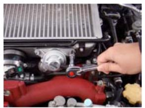
2. Using pliers, carefully clamp onto the spring clamp on the plumb back hose and pull the BOV off the hose. Then carefully remove the clamp completely.
