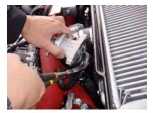
3. Remove the plumb back fitting on the back of the standard BOV and install it onto the Turbosmart BOV using the standard screws.
