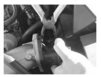
4) Push the plumb back hose onto the plumb back fitting on the new BOV. Use the factory bolts to fit the new BOV onto the intercooler pipe. Remember to install the supplied gasket in between the BOV flange and the intercooler flange. Reinstall the vacuum/pressure source to the nipple. Refit the engine cover. Start the engine and check for leaks.
