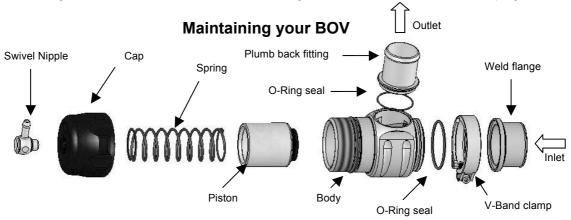
Turbosmart recommends that the following maintenance procedure is carried out at six monthly intervals. Regular maintenance will ensure that your BOV is operating at its peak and will extend the working life of the product.
