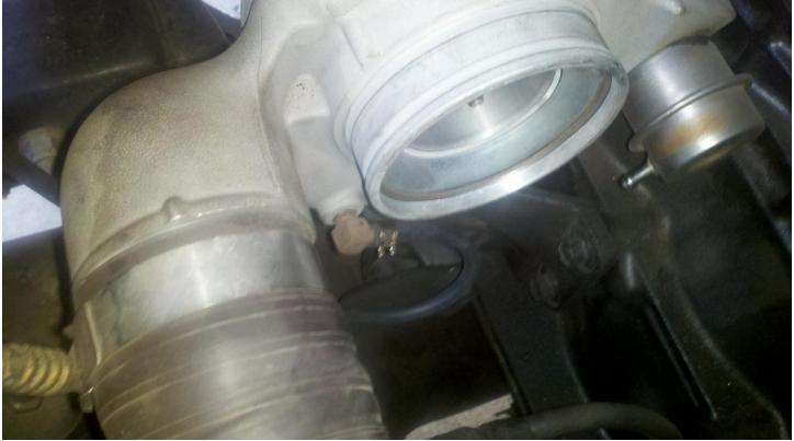
The new actuator can be swapped out quite simply from underneath the truck by removing the factory 6mm nuts and re-using them with the new actuator-
