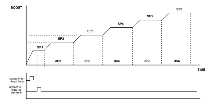
**SSD** (Sequential switching function D): Sequential switching function D is an advanced boost level switching function where you can configure a time delay to give either a drop in boost or a spike between switching boost levels. For example in a drag racing application you may want lower your boost during launch to maintain traction and spike your boost during gear changes to compensate for a drop in RPM.
