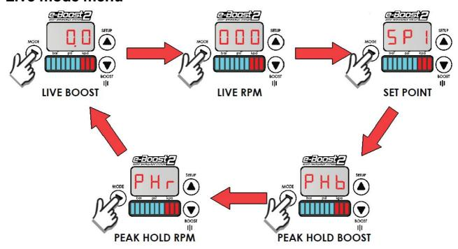
When the e-Boost2 is powered up, the display will automatically go into live mode. Pressing MODE once will scroll through the live mode menu.
