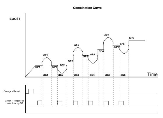
**SSE (Sequential switching function E):** Timed sequential switching function E allows the set-points to be mapped and switched during a predetermined time interval.
