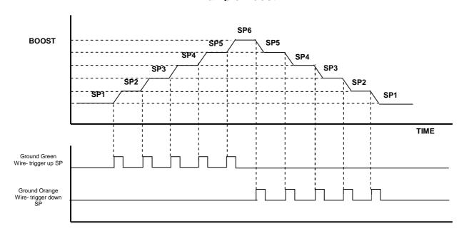
**SSC** (Sequential switching function C): Timed sequential switching function C allows the boost groups/set-points to be active then switched at predetermined time intervals. This switch logic could be applied in a drag racing situation where you want to switch boost levels at known time intervals within your elapsed time (ET).
