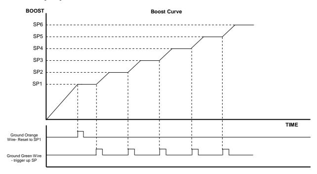
**SSB** (Sequential switching function B): Sequential Switching Function B allows you to sequentially switch up and down between different boost settings using external switches. This switch logic could be applied in a situation where you want to have a different boost levels in each gear.
