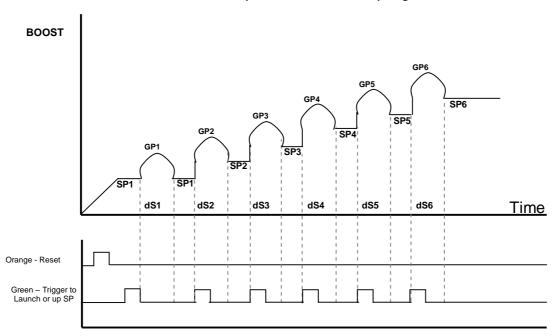
EXAMPLE 3: COMBINATION OF BOOST SPIKING & BOOST DIPPING BETWEEN BOOST LEVEL SWITCHING
