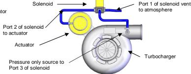
If you are unable to achieve your desired boost pressure, it is normally due to exhaust manifold backpressure forcing the internal waste gate to open. To increase your boost pressure further, fit a higher pressure waste gate actuator to increase your minimum boost pressure.
