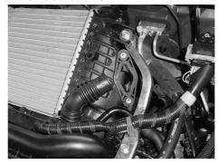
3) Use the factory bolts to fit the new BOV onto the intercooler pipe. Remember to install the supplied gasket in between the BOV flange and the intercooler flange. Reinstall the vacuum/pressure source to the nipple and plumb back pipe to the plumb back fitting and clamp using the factory clamp. Start the engine and check for leaks.
