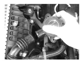
4) Use the factory bolts to fit the new BOV onto the intercooler pipe. Remember to install the supplied gasket in between the BOV flange and the intercooler flange. Reinstall the vacuum/pressure source to the nipple and the plumb back hose. Reinstall the engine cover. Start the engine and check for leaks.
