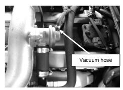
2) Install the Kompact BOV's using the standard bolts. Remember to put in the provided gaskets between the flange and the BOV. Replace the plumb back hose and secure with the standard clamp. Refit the standard vacuum lines and secure with clamps. Start the car and check for leaks.
