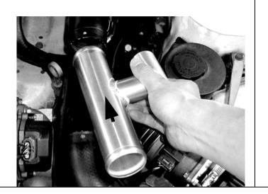
**Step 4.** Use the 70mm new hose clamps supplied to secure the factory hoses to the SR20 Adaptor pipe. Tighten the hose clamps with a 7mm socket or screwdriver.
