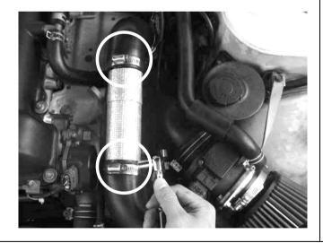
Step 2. Remove the factory pipe.
