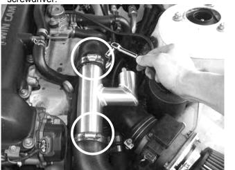
**Step 5.** Locate the intake manifold fitting connected to the factory boost/vacuum line. It is on the left hand side of the engine bay. Remove the factory boost/vacuum line to show the intake manifold fitting.
