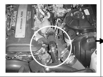
**Step 2.** Loosen the top hose clamp on the factory intercooler pipe.
