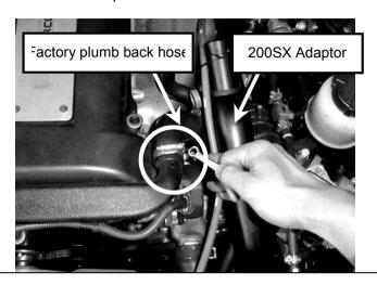
Step 12. Fit the blank-off assembly to the end of the factory BOV return pipe. Secure the blank-off assembly with a 40mm hose clamp supplied.
