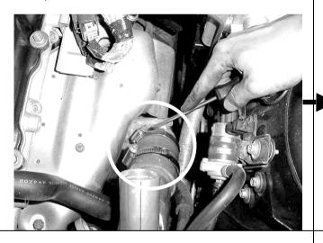
**Step 6.** Use the remaining 60mm hose clamp supplied to secure the intercooler pipe to the 200SX Adaptor pipe. Tighten the hose clamp with a 7mm socket or screwdriver.
