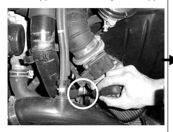
**Step 4.** Fit the Silicon hose coupler over the top of the 200SX adaptor and connect the two ends onto the factory pipes with the BOV mounting pointing towards the rear of the engine.
