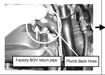
Blank-off Assembly Factory BOV Return Pipe
