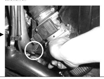
**Step 7.** Locate the Factory BOV under the fuse box on the left hand side of the engine bay. Disconnect the factory vacuum/boost line.
