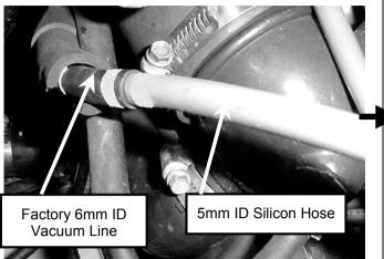
Step 11. Disconnect the factory plumb back hose from the factory BOV return pipe.
