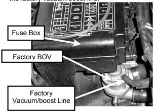
**Step 8.** Take the pre-assembled 5mm ID Silicon hose & reducer and connect the assembly as shown below.
