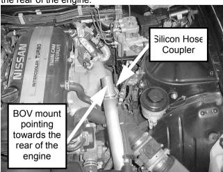
**Step 5.** Use two of the supplied 60mm hose clamps to secure the Silicon hose coupler over the turbo outlet and the 200SX Adaptor pipe. Tighten the hose clamps with a 7mm socket or screwdriver.
