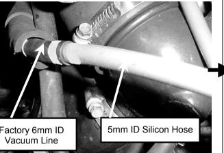
Step 10. Using an 8mm socket or screwdriver, loosen the hose clamp on the factory plumb back hose near the 200SX Adaptor.
