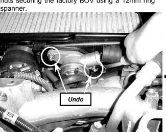
**Step 2.** Remove the hose clamp securing the exhaust hose and disconnect the exhaust hose from the factory BOV.
