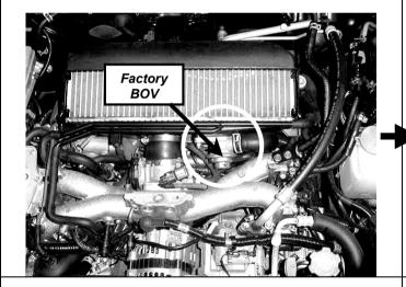
**Step 3.** Disconnect the vacuum/boost line connected to the factory BOV and undo the two nuts securing the factory BOV using a 12mm ring spanner.
