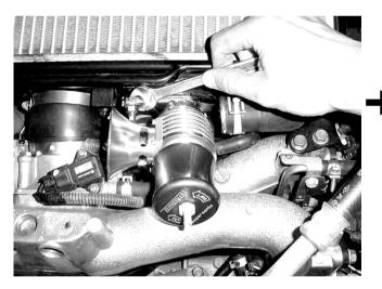
Step 6. Install your Turbosmart BOV onto the adaptor by following your Turbosmart BOV instructions.
