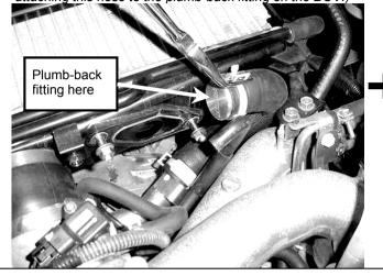
Step 7. Secure the adaptor by fastening the two nuts on either side of the adaptor flange using a 12mm ring spanner.
