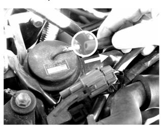
**Step 11.** Undo and remove the two nuts securing the factory BOV using a 12mm socket or spanner.
