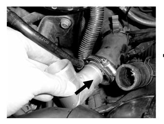
**Step 12.** Release the factory hose spring clamp with a set of long nose pliers and remove the return hose from the factory BOV.
