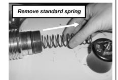
Step 3. Replace your standard spring with the supplied yellow painted atmospheric spring and re-assemble the BOV cap. Refer to the maintenance instructions of your BOV for further information if necessary
