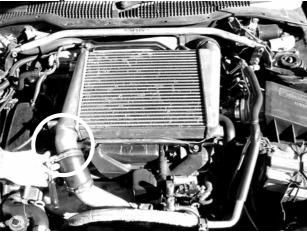
**Step 2.** Undo and remove the 2 bolts on the right hand side of the intercooler cover with a 10mm spanner or socket. Then remove the intercooler cover.
