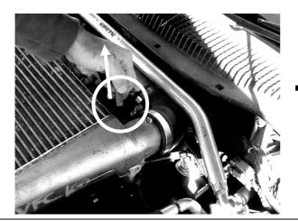
**Step 7.** Undo and remove the 4 bolts on the intercooler bracket with a 12mm spanner or socket.
