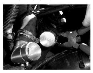
**Step 17.** Install your Turbosmart BOV onto the GTiR Adaptor by following your Turbosmart BOV instructions.
