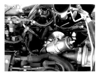
**Step 19.** Remove the four rubber caps on the 4 vacuum fittings on the throttle body.
