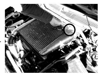
**Step 5.** Disconnect the top intercooler factory boost line from the top right intercooler fitting.
