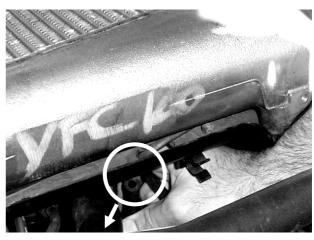
Step 8. Remove the intercooler.
