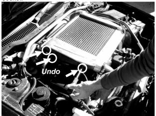
**Step 3.** Using an 8 mm spanner or socket, loosen the bottom factory hose clamp securing the factory hose coupler to the bottom intercooler hose fitting.
