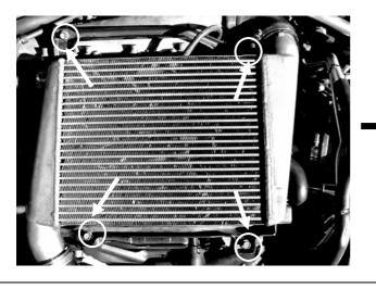
**Step 6.** Disconnect the factory boost line from the bottom right intercooler fitting.
