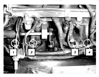
**Step 22.** You will need to use a set of long nosed pliers to access the tight areas around the throttle body. Once fitted, the four vacuum fittings should look the same as the photo below.
