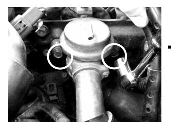
**Step 13.** Undo the factory hose clamp securing the turbo hose to the factory BOV using an 8 millimetre socket. Disconnect the return hose from the factory BOV.
