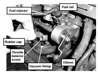
**Step 21.** Connect the numbered ends of the preassembled vacuum hoses to the corresponding throttle body fittings in the previous photo. Secure each vacuum fitting with the 5mm hose spring clamp supplied.
