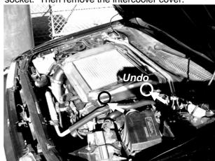
**Step 4.** Using an 8 mm spanner or socket, loosen the top factory hose clamp securing the factory hose coupler to the top intercooler hose fitting.
