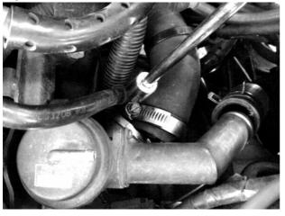
**Step 15.** Insert the 34mm diameter end of the GTiR Adaptor into the factory turbo hose. Secure it with the 50mm constant tension hose clamp supplied using a 7 mm socket or spanner.
