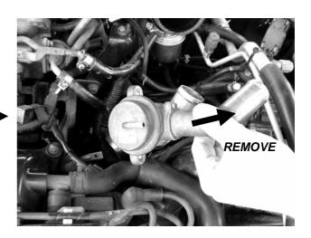
**Step 16.** If using a Dual Port or Plumb Back, go to step 17. Otherwise, blank off the return hose with the 29mm Turbosmart plug supplied. Secure the plug with the factory hose spring clamp.
