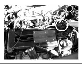
**Step 10.** Disconnect the factory vacuum/boost line from the factory BOV.
