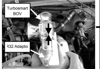
Step 9. Connect the remaining end of the Silicon hose assembly to the Turbosmart BOV fitting. Secure the fitting with the 5mm hose spring clamp supplied.
