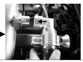
**Step 13.** Connect the Silicon bend to the BOV fitting and factory return pipe. Secure each fitting with a 40mm hose clamp supplied.
