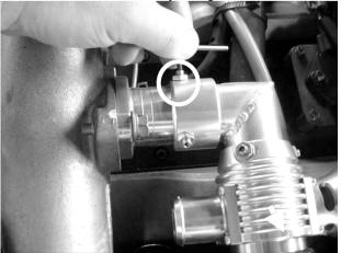
Step 11. Install the R33 Elbow onto the R33 Adaptor.
