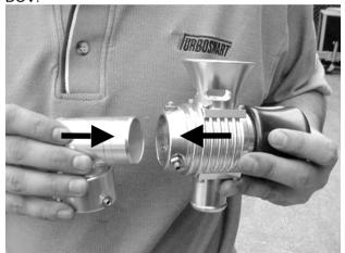
**Step 12.** First loosen the 3 lock nuts using an 8mm socket. Then secure the 3 grub screws onto the R33 Adaptor using a 2.5mm Allen key. Tighten the 3 lock nuts to secure the assembly using an 8mm socket.
