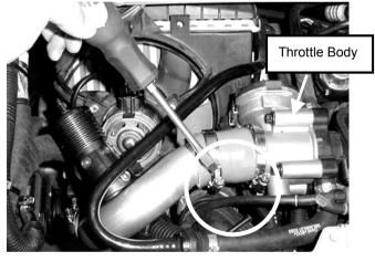
**Step 6.** Install the other Silicon joiner supplied onto the throttle body and secure it with a 50mm hose clamp. Then fit the right hand side of the Smartcar adaptor onto the throttle body Silicon joiner.
