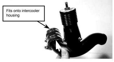
**Step 7.** Tighten the two 50mm hose clamps supplied on the throttle body side with a 7mm socket or screwdriver.
