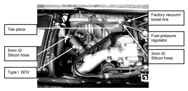
**Step 12.** Ensure there is adequate clearance around the BOV allowing for engine movement and that the BOV does not interfere with the intercooler cooling fan.
