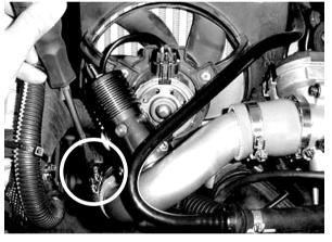
Step 9. Remove the factory boost/vacuum line to expose the fuel-pressure regulator fitting.
