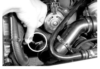
**Step 3.** Remove the factory pipe and rubber sleeve on the throttle body.
