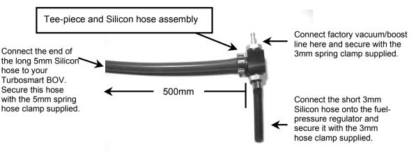
**Step 11.** When installed, the fully assembled tee-piece connection should look the same as the diagram below.
