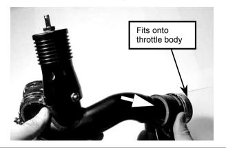
**Step 8.** Tighten the two remaining 50mm hose clamps supplied on the intercooler side with a 7mm socket or screwdriver.
