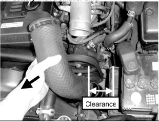
**Step 19.** Fit the adaptor between the intercooler and the throttle body. Using two of the 90mm hose clamps supplied, secure the Silicon hose coupler onto the Soarer adaptor and the throttle body.
