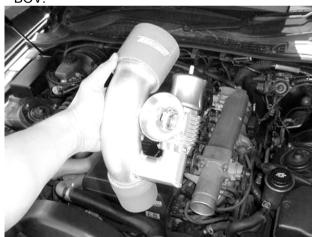
**Step 20.** Using two of the 70mm hose clamps supplied, secure the Silicon hose coupler onto the Soarer Adaptor and the intercooler pipe.
