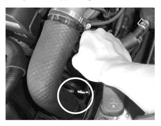
Step 17. Remove the factory intercooler pipe. Important! You may need to increase the clearance between the Soarer TT adaptor and car battery to accommodate for the BOV. To increase the clearance you may have to adjust or replace the car battery with a smaller unit.
