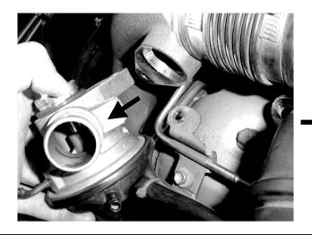
**Step 11.** Block off the factory return hose with the 29mm blanking plug supplied. Use the supplied 40mm hose clamp to secure the plug. Then tighten, using a 7mm socket.
