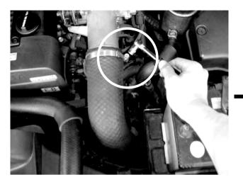
**Step 16.** Undo the hose clamp on the bottom of the factory intercooler pipe, using a 10mm socket.
