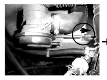
**Step 4.** Undo the hose clamp on the factory BOV return pipe using an 8mm socket. Then disconnect the return pipe from the BOV.
