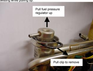
2. Push the fuel rail adapter into the fuel rail and replace the retaining clip.
