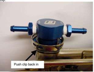
3. Connect the outlet port of the adapter to the FPR fuel inlet port. Connect the return port of the adapter to the FPR fuel outlet port.
