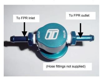
4. Your FPR should be connected to the fuel rail adapter as shown
