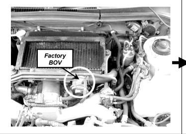
**Step 2.** Using a 12mm socket or spanner, undo the two nuts securing the factory BOV. Remove the hose clamp securing the return hose and disconnect the return hose from the factory BOV.
