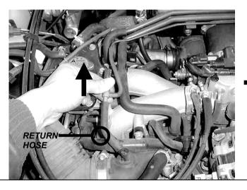
**Step 12.** Reconnect the plastic reducer to the return hose feeding back into the big air intake pipe.
