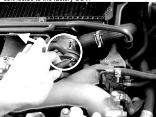
**Step 4.** Remove the factory BOV and old factory gasket.
