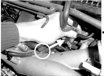
**Step 9.** Install one end of the Silicon hose assembly supplied onto the intake manifold fitting and secure with the 6mm spring clamp supplied.
