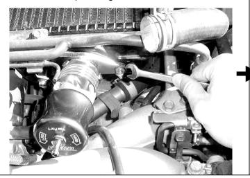
**Step 15.** Insert the free end of the Silicon hose assembly over your Turbosmart BOV fitting and secure it with the 5mm hose spring clamp supplied.
