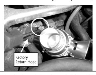
**Step 18.** Secure the boost hose to the BOV and the intercooler fitting using the factory hose clamps.
