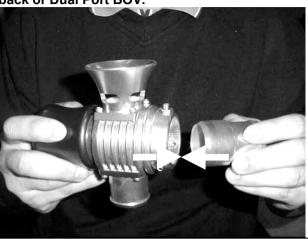
**Step 13.** Connect the remaining end of the Silicon hose assembly onto the BOV and secure it with the 5mm spring clamp supplied.
