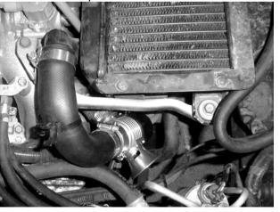
**Step 16.** Connect the plumb back fitting to the factory return hose and secure using the factory hose clamp.
