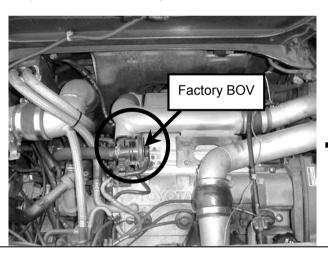
**Step 3.** Disconnect the two vacuum/boost lines from the factory BOV.
