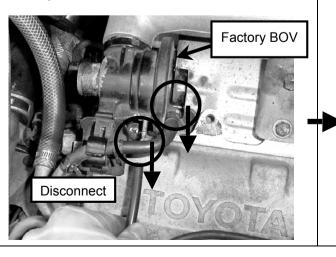
**Step 4.** Using a 12mm socket or spanner, loosen the factory bolt securing the factory BOV to the pipe flange.
