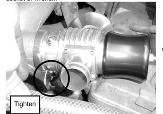
**Step 15.** Connect the factory vacuum/boost hose to the Turbosmart BOV fitting. Secure the fitting with the 5mm spring clamp supplied. Your installation is complete.\_\_\_\_\_
