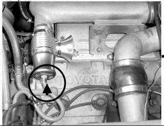
**Step 13.** Install the BOV and MR2 adaptor assembly, secure the adaptor with the factory bolt using a 12mm socket or wrench.
