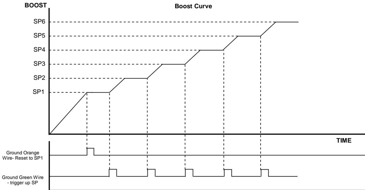
**SSB (Sequential switching function B):** Sequential Switching Function B allows you to sequentially switch up and down between different boost settings using external switches. This switch logic could be applied in a situation where you want to have a different boost levels in each gear.
