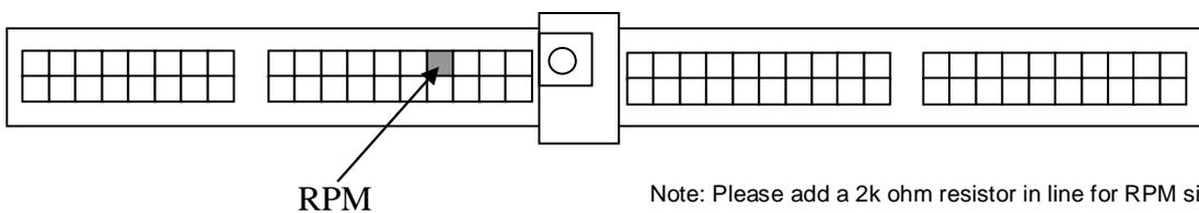
Note: Please add a 2k ohm resistor in line for RPM signal
