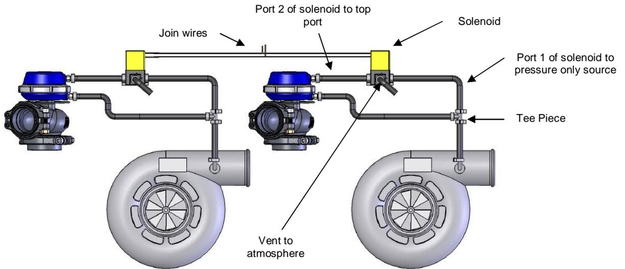
**Two port, single solenoid, single turbo connection Method (2)**
