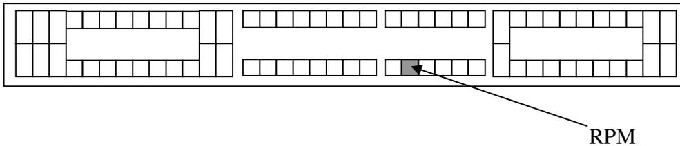
**Note:** For your rpm signal to work correctly with this ECU you may need to place a 3.3K ohm ¼ watt resistor (Colour code: orange, orange, orange, gold) in series with the yellow rpm input wire before connecting to the ECU.
