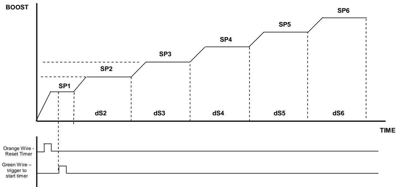
**SSD (Sequential switching function D):** Sequential switching function D is an advanced boost level switching function where you can configure a time delay to give either a drop in boost or a spike between switching boost levels. For example in a drag racing application you may want lower your boost during launch to maintain traction and spike your boost during gear changes to compensate for a drop in RPM.
