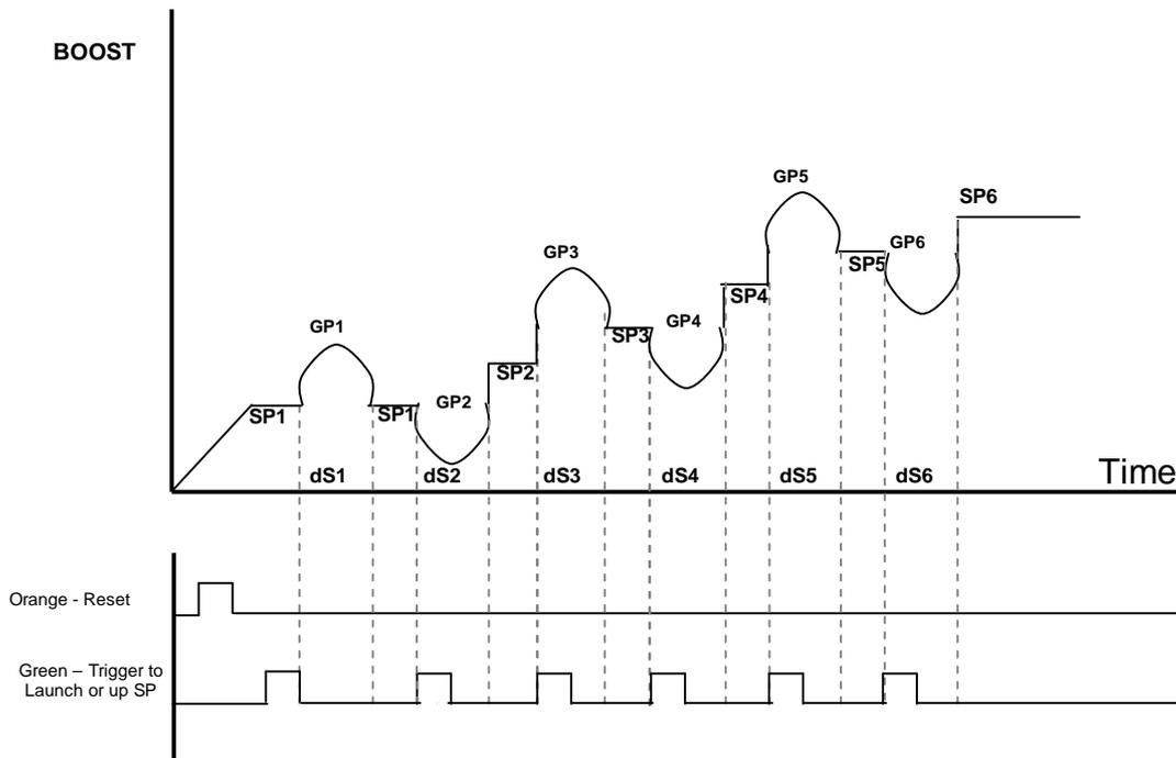
**SSE (Sequential switching function E):** Timed sequential switching function E allows the set-points to be mapped and switched during a predetermined time interval.
