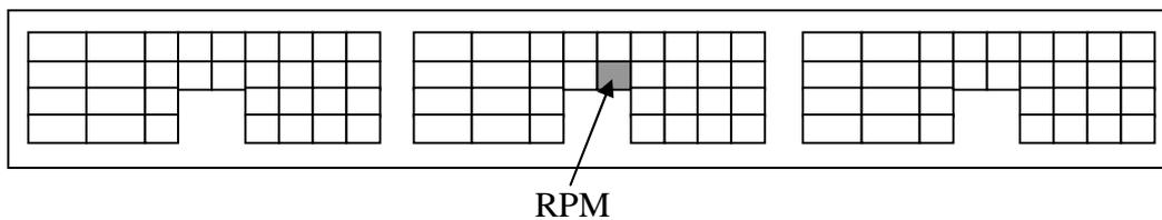
**Note:** For your signal to work correctly with this ECU you will need to place a 2K ohm ¼ watt resistor (Colour code: red, black, red, gold) in series with the yellow rpm input wire before connecting to the ECU.
