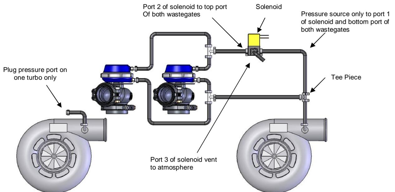
**Two port, twin solenoid, twin turbo connection Method (1)** (For controlling boost on a twin turbo, twin wastegate, twin solenoid turbo system, on a V configuration engine with high back pressure)
