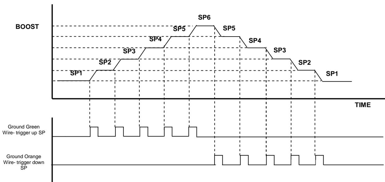
**SSC (Sequential switching function C):** Timed sequential switching function C allows the boost groups/set-points to be active then switched at predetermined time intervals. This switch logic could be applied in a drag racing situation where you want to switch boost levels at known time intervals within your elapsed time (ET).
