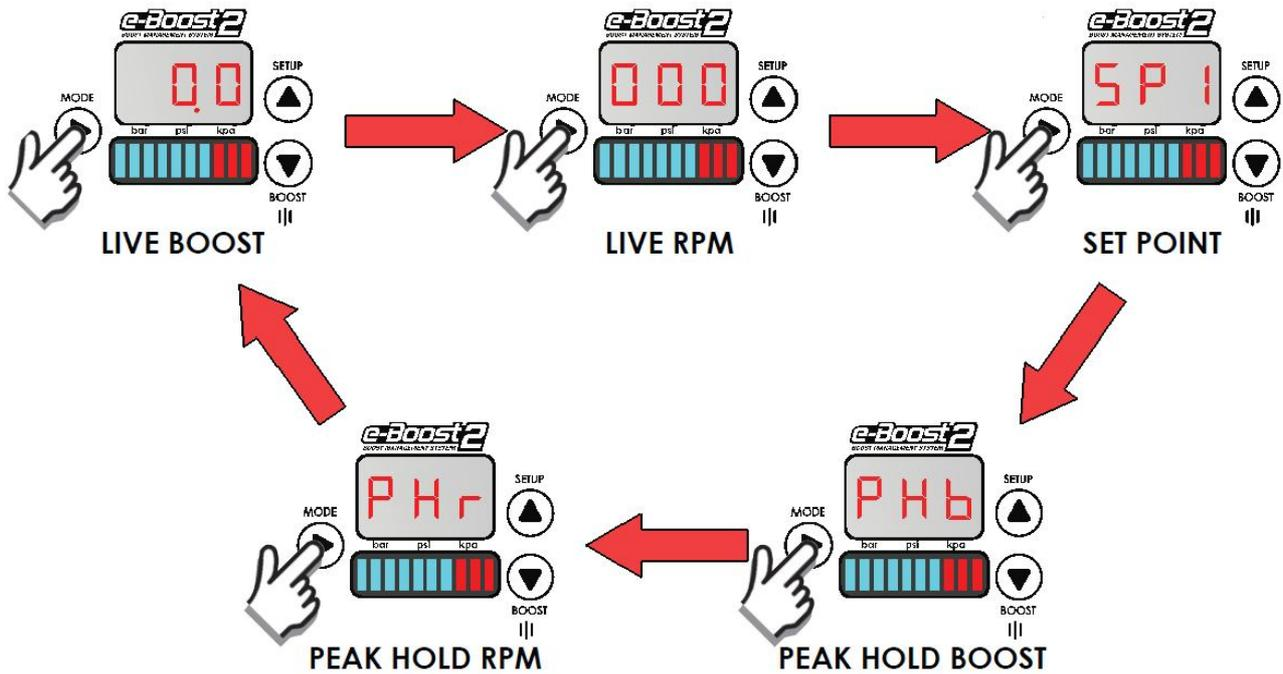
When the e-Boost2 is powered up, the display will automatically go into live mode. Pressing **MODE ONCE** will scroll through the live mode menu.
